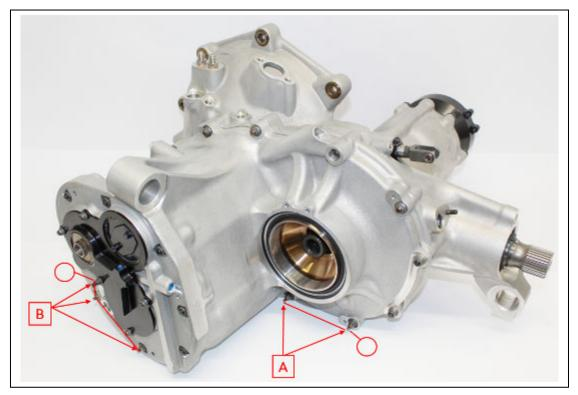
A / B = FIA sealing tag + 2 aluminium seals C = 2 aluminium seals
