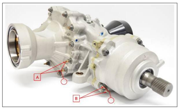
A / B = FIA sealing tag + 2 aluminium seals C = 2 aluminium seals
