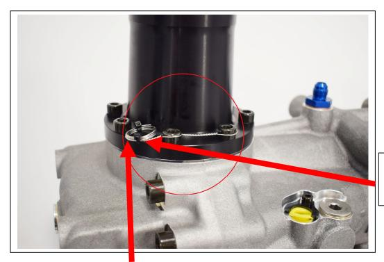
Aluminium seal (max 20mm from the screw)
